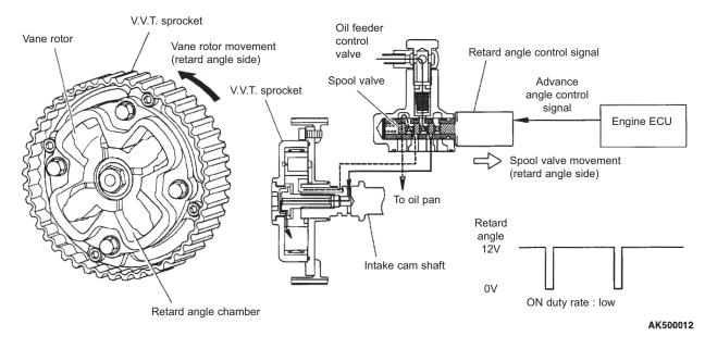
• The oil feeder control valve spool valve travels in the retard angle direction on a retard angle control signal from the engine ECU.
