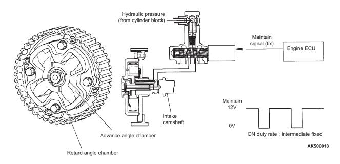
When the actual phase angle reaches the target phase angle, the advance angle chamber and retard angle chamber hydraulic pressures are maintained, as is the phase angle of the intake cam shaft. When this happens, the oil feeder control valve is controlled so that the actual phase angle is same as the target phase angle.
