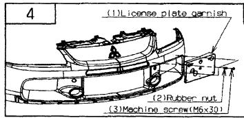
Front bumper Section (3) Machine screw (2)Rubber nut (after tightening) (before tightening
