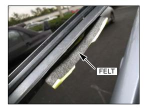
4. Remove the liner from the back of the felt pieces. Affix the felt on the inner clips as shown.
