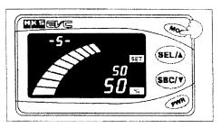
(1) In monitor mode, hold the (MOD) button down (for more than 1second) and press (MOD) 1 more time. The top left corner should display a "-5-".
