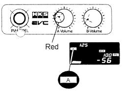
(13) To select between mode A and mode B, press the (PWR/SEL) switch once (short press). The selected volume knob will light up red. Example: The diagram shows when the mode A boost setting is selected.
