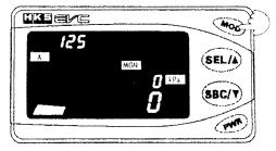
(3) Add 10kPa to the higher boost setting between mode A and mode B.
