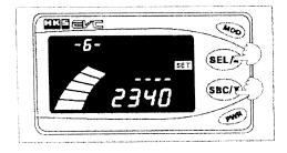
(2) Use the (SEL/ $\triangle$ ) or (SBC/ $\nabla$ ) button to input the lock code number.
